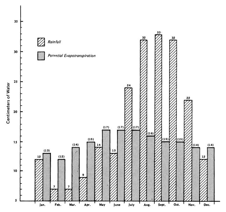
Figure 1.—Rainfall and potential evapotranspiration data at Agana, as calculated by the modified Thornwaite method (3).
