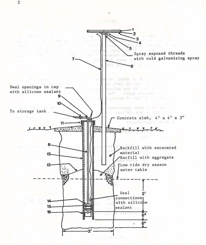
Figure 1. Assembly drawing of the "WERI Well" (not to scale). Refer to Table 1 for a descriptional of parts of the well.
