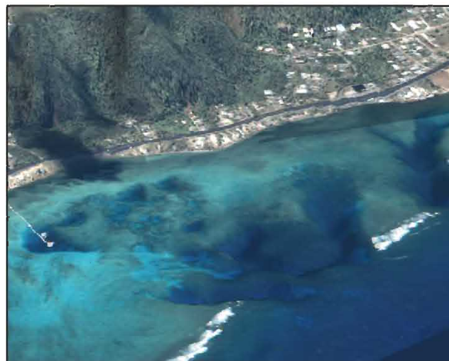
Figure 15. 3-D model of the Piti Bomb Holes Marine Preserve created by "draping" pan-sharpened IKONOS satellite imagery over digital bathymetry data collected from an airborne LIDAR sensor. IKONOS imagery copyright of Space Imaging LLC.
