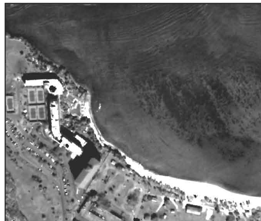
Figure 12. A panchromatic IKONOS image of the coastal area near Ypao Beach in Tumon Bay, Guam. Panchromatic IKONOS images are composed of a single, black and white band and have a spatial resolution of 1 meter. Image copyright of Space Imaging LLC.
