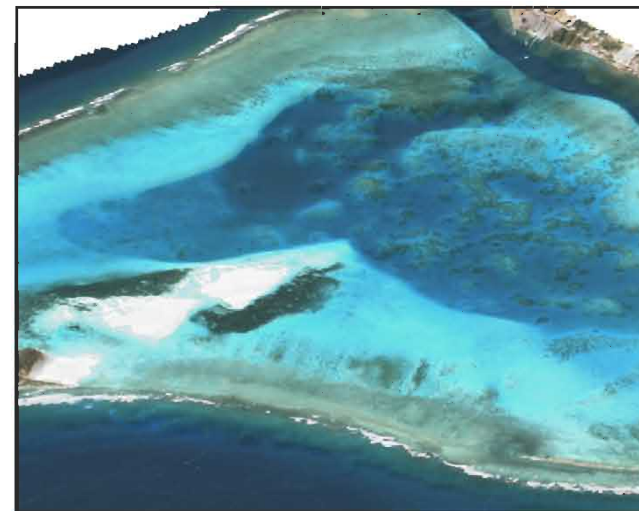
Figure 16. 3-D model of Cocos Lagoon created by "draping" pan-sharpened IKONOS satellite imagery over digital bathymetry data collected from an airborne LIDAR sensor. IKONOS imagery copyright of Space Imaging LLC.
