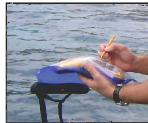
Figure 4. A hand-held Trimble GeoXT GPS receiver used to record a position near Pati Point, Guam. Photo by John Tomczuk.
