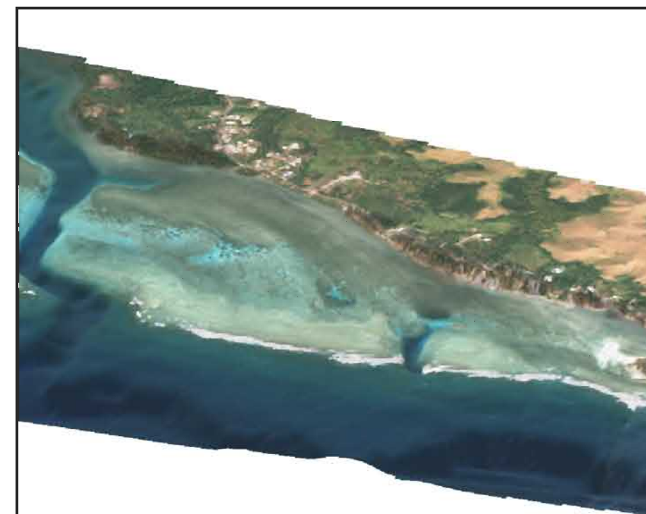
Figure 17. 3-D model of the Achang Reef Flat Marine Preserve created by "draping" pan-sharpened IKONOS satellite imagery over digital bathymetry data collected from an airborne LIDAR sensor. IKONOS imagery copyright of Space Imaging LLC.
