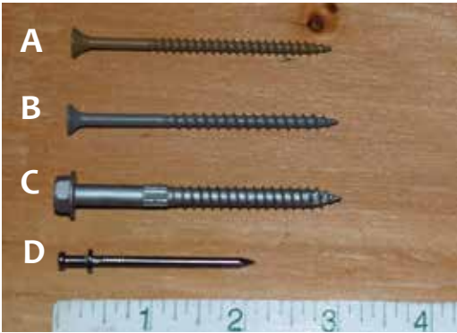
Figure 2.23. Key materials for fastening plywood panels include (A,B) 3 inch wood driving screws that allow a 2 inch embedment, (C) ¼ lag screw that is three inches long, (D) duplex or two-headed 2-inch nail. Source: University of Hawaii Sea Grant.
