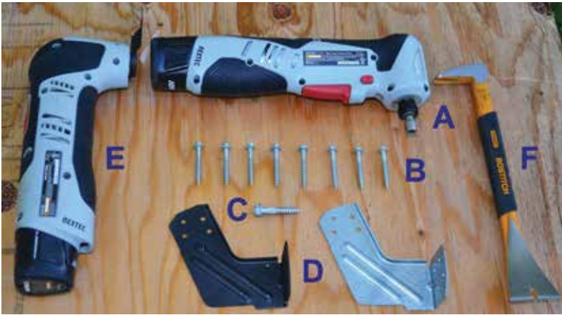
Figure 2.18. In an installation where the molding needs to be removed, it is easily done with a multi-tool (E) and a nail-trim remover (F).
