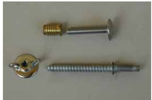
Figure 2.25. Another method uses brass grommets screwed into the wood frame. A wide head screw attaches the panels. The lower screw and washer wing nut are used to hold the top two corners. Source: University of Hawaii Sea Grant.
