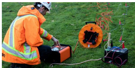
Electrical Resistivity Tomography, subsurface imaging analysis example (from Terradat®)
